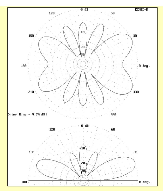
On 17, the two patterns return to close coincidence. Whether patterns are similar or different will vary with feedline length and dress, as well as frequency.
