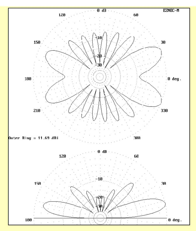
Although your situation is unlikely to copy this one, studying the upper and lower patterns for each band may give you a better idea of how to compare the details of antenna patterns.
