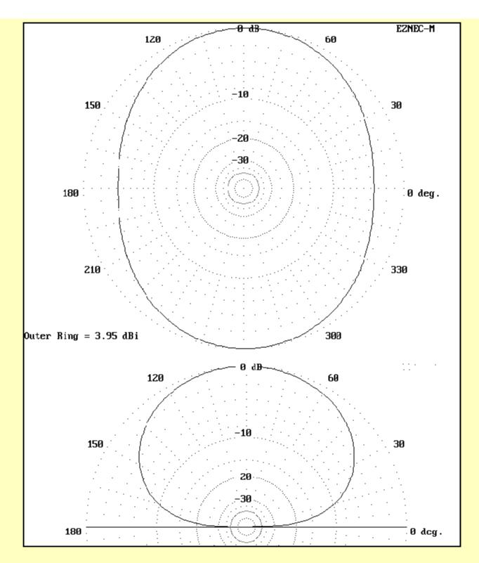
Note: Since the actual elevation angle of maximum radiation is greater than 45 degrees, the azimuth patterns are taken at an elevation angle of 45 degrees.
