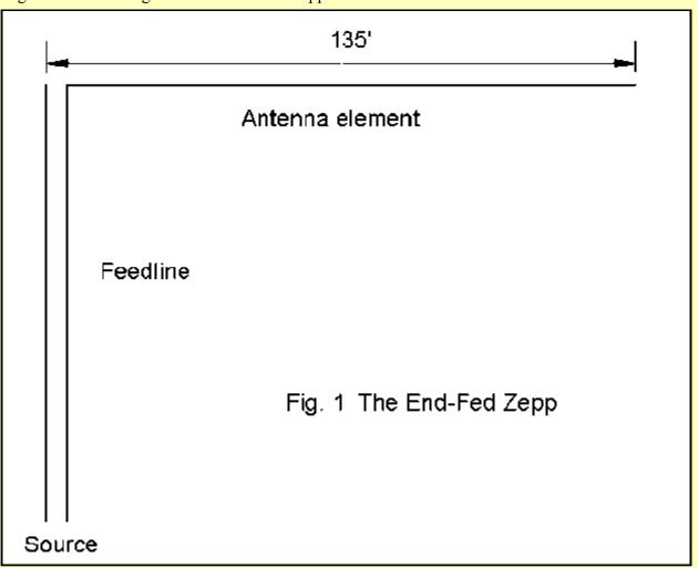
The Zepp can be cut for other bands, but a 135' length of #14 wire at a height of about 35' is one of the most common ham installations. 35' is only about 1/8 wavelength at 80 meters and about 1 wavelength at 10 meters. Therefore, the Zepp will exhibit all the variability and sensitivity to terrain of any low horizontal antenna.
