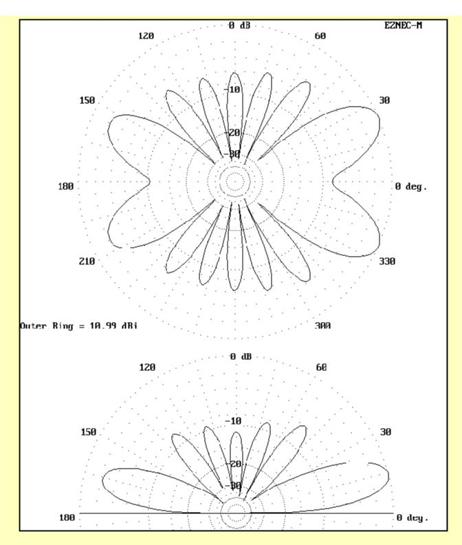
Note how slight thickening of the elevation lobes produces a significant decrease in the maximum gain of the main lobes of the pattern.
