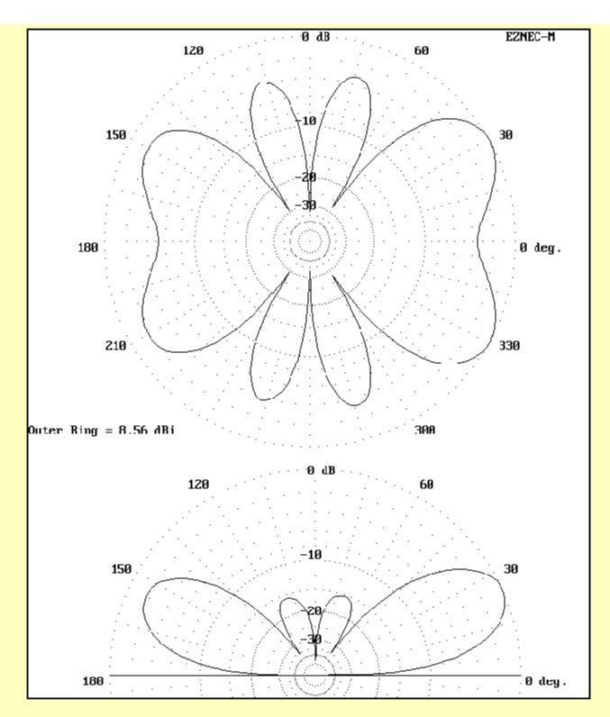
The feedline radiation below significantly rounds all the lobes of the azimuth pattern and reduces maximum gain while increasing overall broadside radiation.
