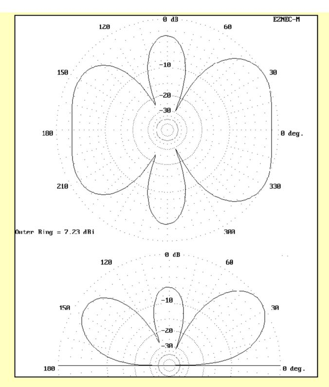
Note that at this frequency, the feedline radiation actually lowers the elevation angle of maximum radiation, a fairly rare occurrence with shorter lengths of feedline.
